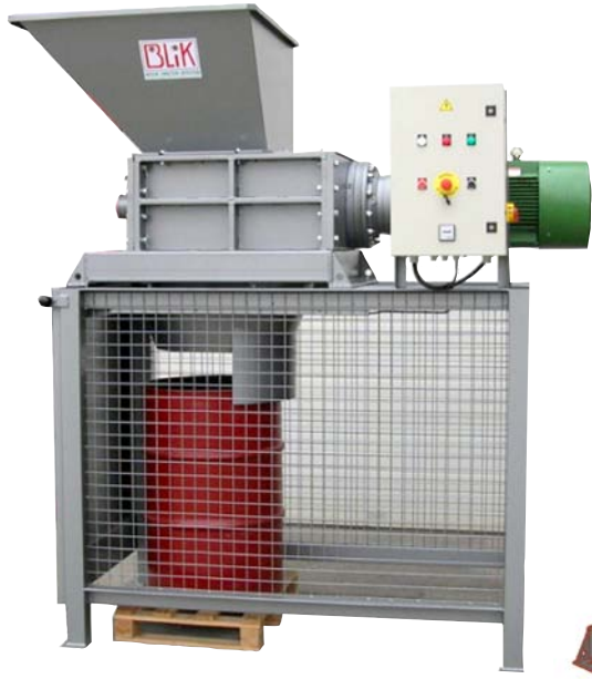
BLiK B600 crusher: destruction of pallets
