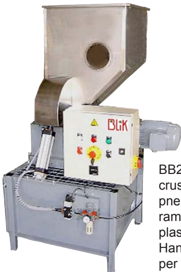
BLiK crusher BB160 destruction of tickets and plastic cards
