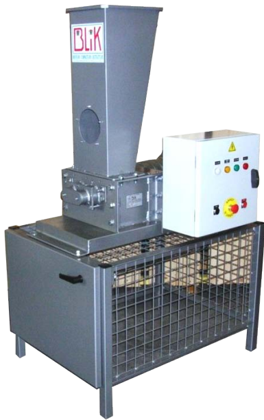
BLiK crusher BB160 destruction of tickets and plastic cards
