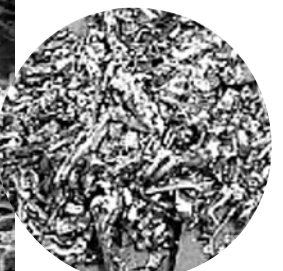
Crushing "carrots" from a zinc alloy foundry (huge reduction in volume, reprocessing).
