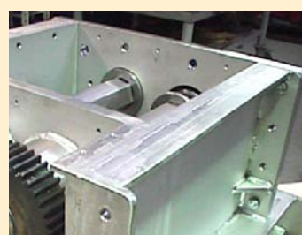
Stainless steel: cutting block without blades.
