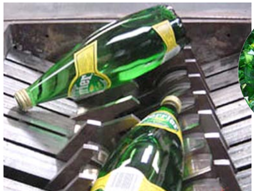
Crushing glass bottles in a BLiK B400 crusher, equipped with glass breaking blades.
