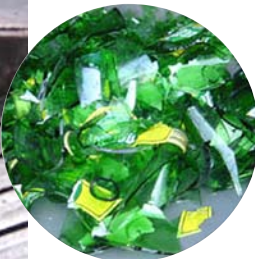
Agro alimentary: shredding of plastic moulds (here, yoghurt containers) in a BLiK shredder: total amount divided by 10
