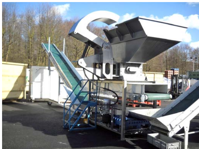
B600-510 + Q500-510 crushing of joints automobile rubber
