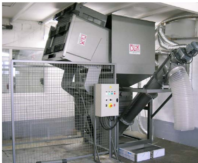
B400-510 Crusher with raise-container and screw of liquid-solid separation
