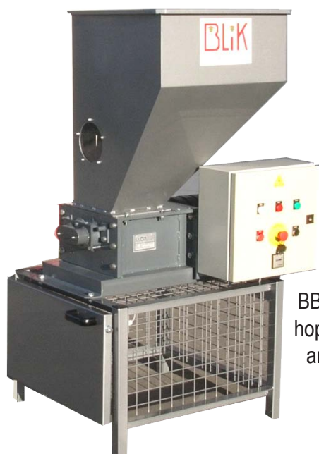
BB230 BLiK crusher: with pneumatic rammer: for plastic bottles. Handles 500-600 per hour.
