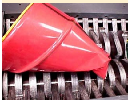
Crushing metal containers in a BLiK B600
