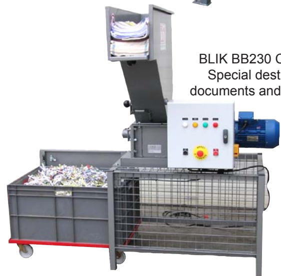
BB230 with output «BLIK endless screw» filling bag upright
