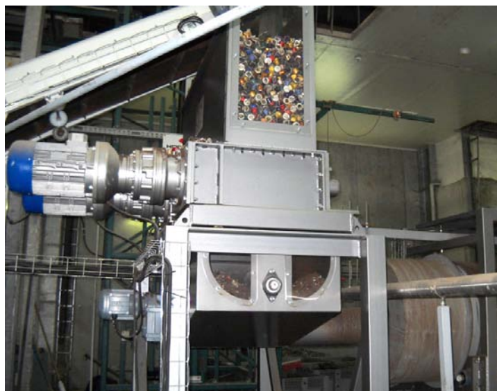
B400-510 crushing of coffee dosettes + separation aluminum and coffee + rinsing
