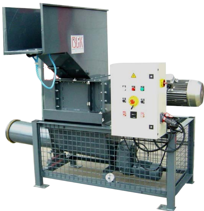
Crusher BLiK B400 output endless screw
