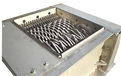
Stainless steel: cutting block and blades.
