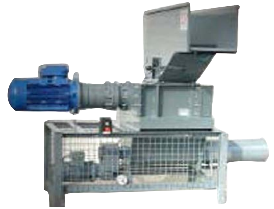
BLiK crusher, special "fireproof" version for petrol tanks
