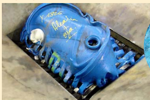
Crushing plastic containers in a BLiK B600.
