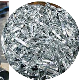
Shredding galvanised tubes in a BLiK shredder (huge reduction in volume, reprocessing).
