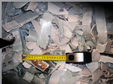
After magnetic sorting by overband : the plastic
