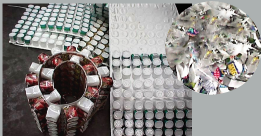
Agro alimentary: shredding of plastic moulds (here, yoghurt containers) in a BLiK shredder: total amount divided by 10
