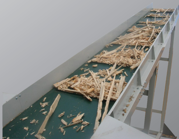
Wood evacuation after separation of the metallic points.
