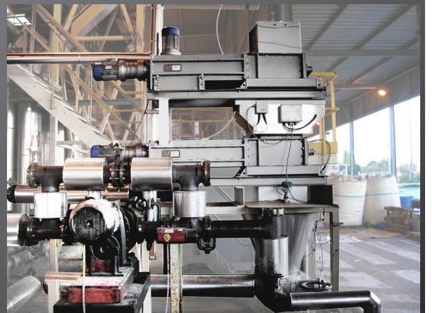
B400-510 grinding of hot bitumen
