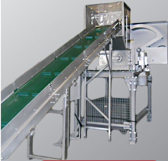
BLIK B600 Crusher with load by conveyor and electric arm
