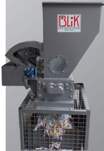
BLIK crusher BB160 destruction of tickets and plastic cards
