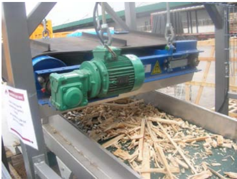
magnetic separation of the points
