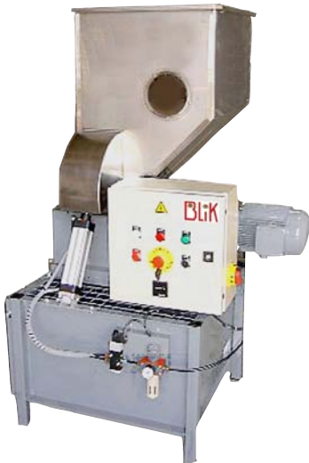
BB230 BLiK crusher: with pneumatic rammer: for plastic bottles. Handles 500-600 per hour.
