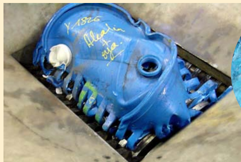
Crushing plastic containers in a BLiK B600.
