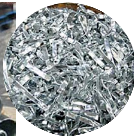
Shredding galvanized tubes in a BLiK shredder (huge reduction in volume, reprocessing).
