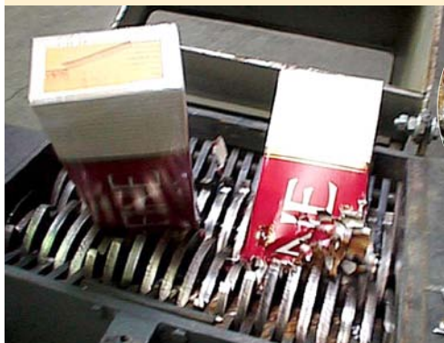
Administration, police, justice: destruction of seized goods for legal reasons: solution: a "universal" BLiK shredder (here, packets of cigarettes).
