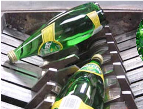
Crushing glass bottles in a BLiK B400 crusher, equipped with glass breaking blades.
