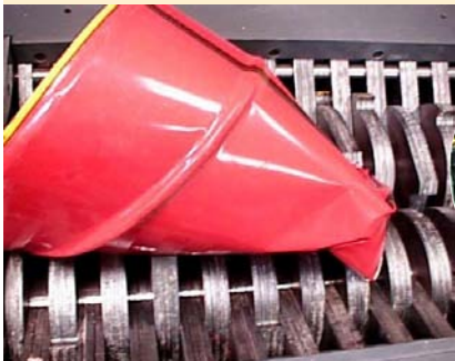
Crushing metal containers in a BLiK B600
