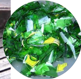
Agro alimentary: shredding of plastic moulds (here, yoghurt containers) in a BLiK shredder: total amount divided by 10
