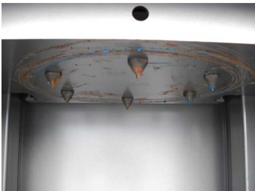
punches for the maintenance of the barrel and the emptying of the air
